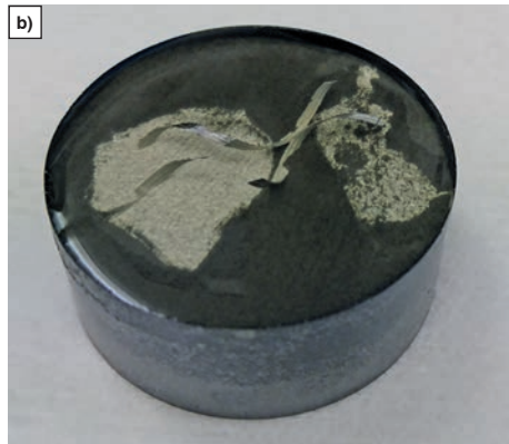
Figs. 6a and b: a) Sample cold mounted in epoxy resin with subsequently made contact (e. g. screw); b) cold mounted sample, additional hot mounting to realize conductivity.
