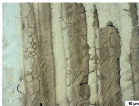
Fig. 30: Magnesium alloy, electrolytically polished with acetic acid-based electrolyte, unetched; bright field.
