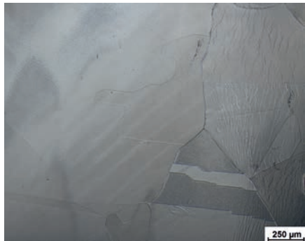
Fig. 3: Electrolytically polished sample made of pure indium (raw material: TU Freiberg).
