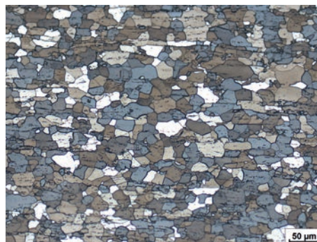
Fig. 39: Grade 4 titanium, electrolytic preparation, etching according to Keller and then color etching according to Weck; bright field.
