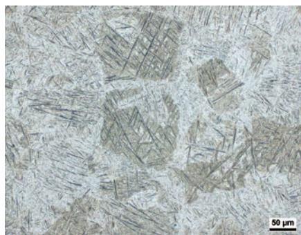
Fig. 34: TiAl6V4, mechanical preparation, core structure, etching: Kroll; bright field.
