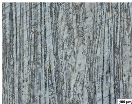
Fig. 29: Magnesium alloy, electrolytically polished with perchloric acid base, etching with aqueous electrolyte content.
