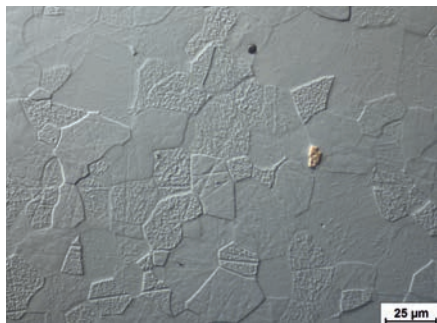
Fig. 15: Ferritic steel, mechanical preparation, unetched, very fine deformations still visible, non-metallic inclusions remain, preparation time > 30 min; DIC.
