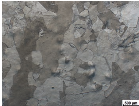
Fig. 4: Battery lead, electrolytically polished. The wavy surface structure is a characteristic of electrolytic preparation.
