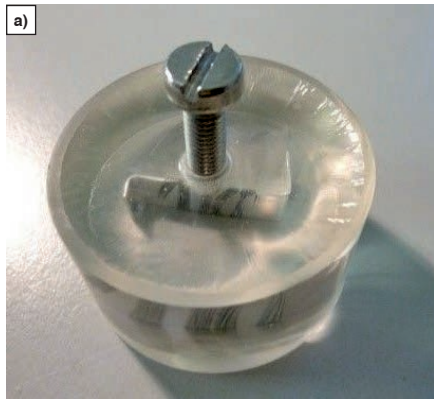
Figs. 6a and b: a) Sample cold mounted in epoxy resin with subsequently made contact (e. g. screw); b) cold mounted sample, additional hot mounting to realize conductivity.
