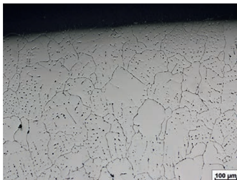
Fig. 14: Aluminium, electrolytic preparation, unetched, possibly more pronounced edge rounding at longer polishing times, bright field.
