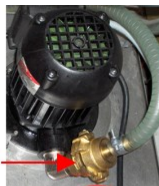
A Pump outlet
