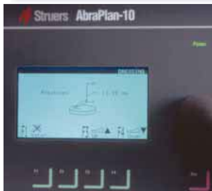
The operator can monitor the thickness of the stone through its entire lifetime
